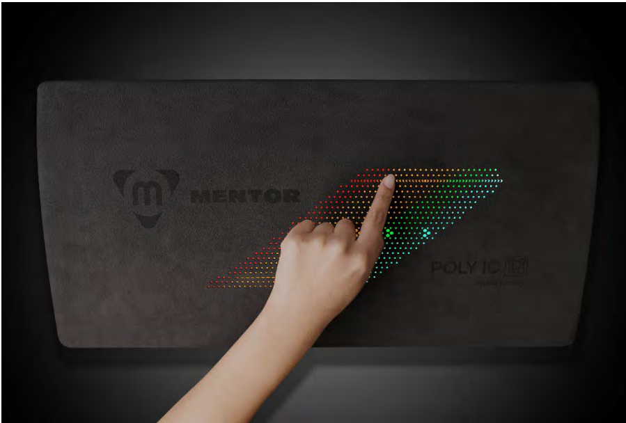
Pic. 3: Use the touch function in the centre of the light surfaces to select individual segments. At the top of the demonstrator, you can then set the colour, while the brightness can be continuously adjusted at the bottom.
